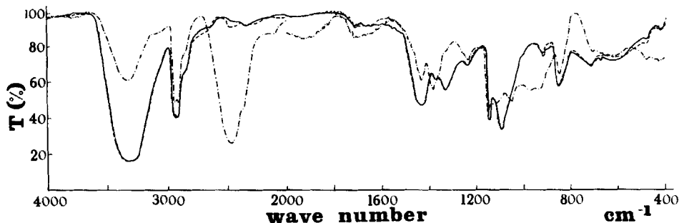
FIG. 3. IR spectra of PVA: nondeuterated (—), deuterated (— · —), and after substituting deuterium for hydrogen (— —).
